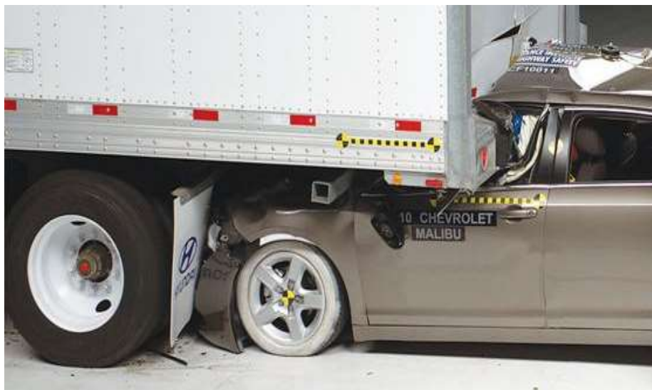
Figura 2.16 Prueba de choque trasero del Insurance Institute for Highway Safety [IIHS, 2011]
